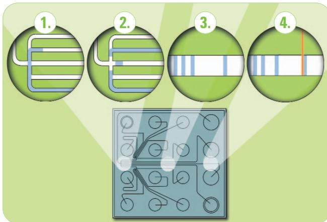
1. The sample moves through the microchannels from the sample well.
